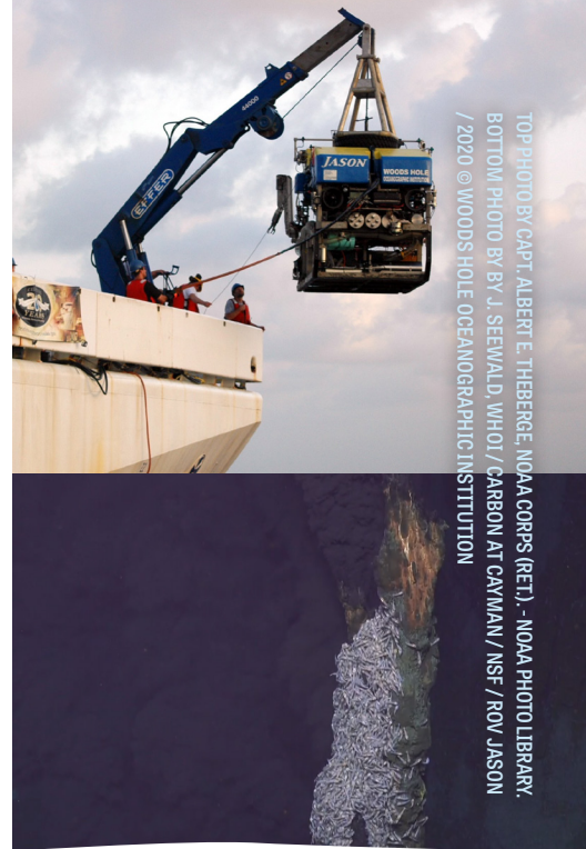
Top: Woods Hole Oceanographic Institution's submersible ROV (remote operated vehicle) "Jason," used for studying deep sea hydrothermal vents. Bottom: Shrimp cluster on a hydrothermal vent.
