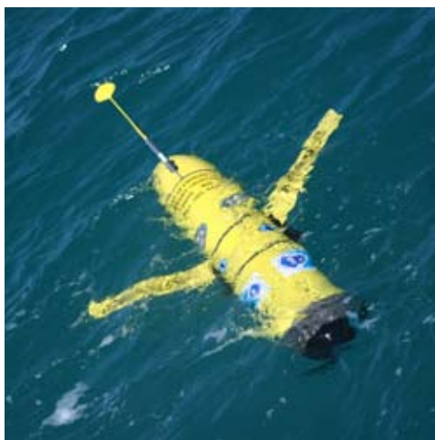
The above picture shows a Slocum Glider, also referred to as an Autonomous Underwater Vehicle (AUV). The glider is designed to monitor area waters at varying depths in order to detect harmful algal blooms and the conditions under which they form.
