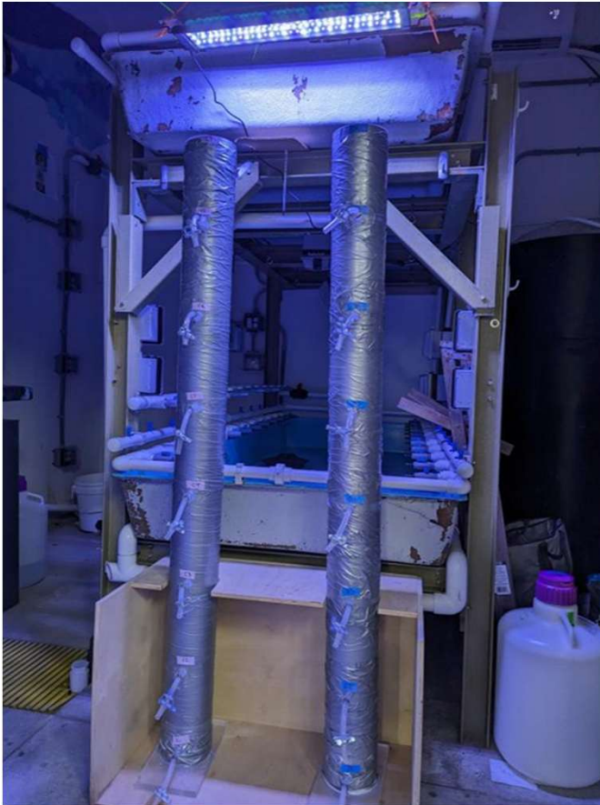
Figure 1. Experimental set up showing the control and treatment columns in support apparatus with light source above. Columns are shrouded in brown craft paper over which is wrapped duct tape.
